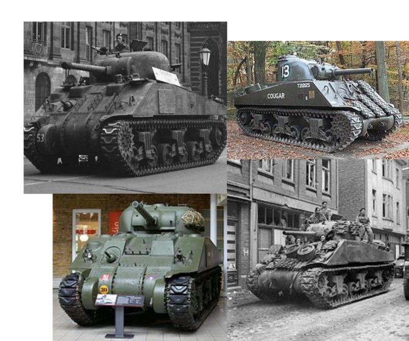
Туре Medium tank Place of origin **United States** July 1942 – November 1943 Produced No. built 7,499 Specifications Mass 31.6 tonnes (67,000 lbs) Length 6.06 m (19 ft 11 in) Width 2.62 m (8 ft 7 in) 2.74 m (9.0 ft) Height Crew 5 13–76 mm (0.5–3.0 in) Armor Main Armament 75 mm M3 L/40 Gun 97 rounds Secondary Armament 1×.50 cal Browning M2HB machinegun 300 rounds 2×.30-06 Browning M1919A5 machineguns 4,750 rounds Engine Chrysler A57, 30 cylinder gasoline
